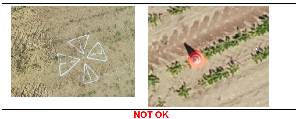
Figure 2: Improper GCP markers
